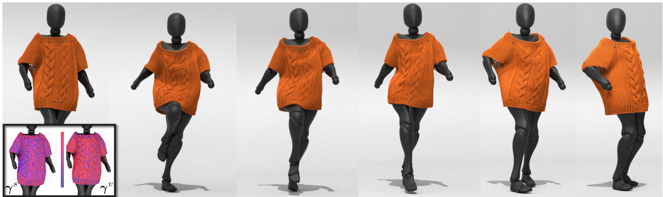
Fig. 1. Yangge dance. We propose a volumetric homogenization algorithm for knitwear simulation. Our pipeline takes full-scale yarn-level simulation observations as input and learns a homogenization out of the input poses. We name this procedure volumetric-homogenization because we do not homogenize yarn-level dynamics to a codimensional sheet/shell domain but to a volumetric enclosure. Doing so allows us to use an intuitive hyperelastic material model with a volume-preserving constraint to capture nonlinear behaviors like bending and twisting. volumetric homogenization varies spatially. Each volumetric element has its own material parameter, which substantially enhances the expressivity of our model. This is a challenging problem, we utilize the adjoint Gauss-Newton method[Zehnder et al. 2021] to enhance the convergence of the adjoint method. Additionally, we propose harmonic initialization, sample-based optimization, and a novel domain-decomposed projective dynamics solver, which significantly accelerates the entire optimization process. In the teaser figure, we show snapshots of an animated virtual character performing a Yangge dance, where we simulate a homogenized tetrahedron mesh with about 390K elements that encapsulate a sweater. Cable patterns on the garment contribute to an irregular and sophisticated material distribution (as visualized in the sub-figure). In this example, the mesh-level simulation runs at 604 ms per frame on average under \Delta t = 1/150 sec. The yarn-level sweater model, on the other hand, consists of over 3M DOFs. Our volumetric homogenization makes the simulation \sim 100\times faster than simulating the sweater at the yarn level.
