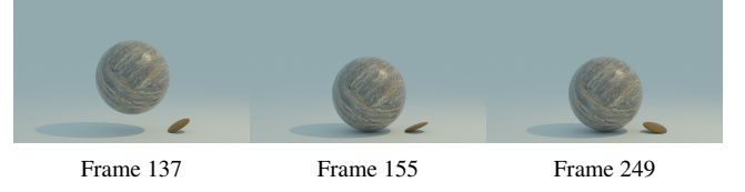
Figure 5: Falling ball with lower resolution LBM. The coin inaccurately adheres to the ground during the sphere’s descent. This experiment used a resolution of 200 \times 360 \times 400 , with a runtime of 2.6 seconds per frame.
