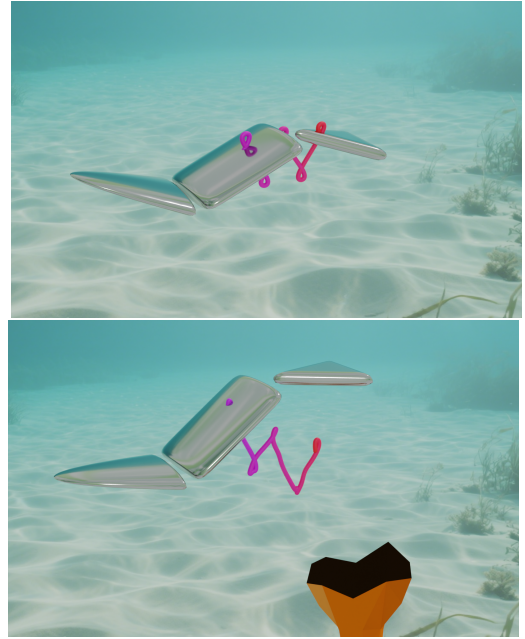
Figure 9: The impact of a large oscillating fish tail on the robotic fish's movement, showing significant lateral drift caused by fluid interaction. The original and disturbed trajectories are shown in red for comparison.
