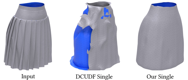
Fig. 8. Example of single layer extraction: DCUDF cannot produce valid single layers using graph cut with smooth energy only, while our method can extract the single layer mesh with the same resolution of 32^3 .
