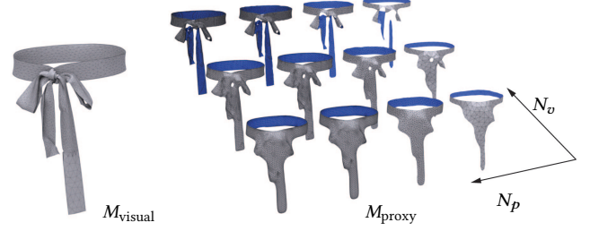
Fig. 5. Voxelization resolution N_v and target proxy mesh vertex count N_p : N_v from front to back, 32, 64, and 128, controlling the details and categorization of single layers. N_p from right to left, 128, 1024, 8192, and 65536, controlling the desired size of the uniform mesh.
