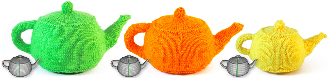
Fig. 15. Knitted teapots with different numbers of stitches using different knittable stitch meshes generated from the same input mesh in Fig. 1. They are all knitted using 6 separate yarn pieces and they contain 6.3K, 4.4K, and 2.6K stitches from left to right.
